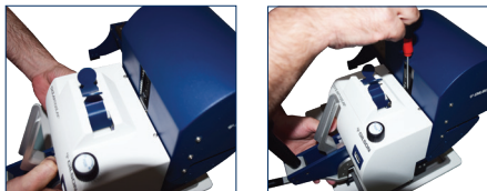
Figure 6 Pull the head down a little and turn the screw to the lower stop
