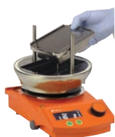
Insert the adapter into the GreenHouse base
