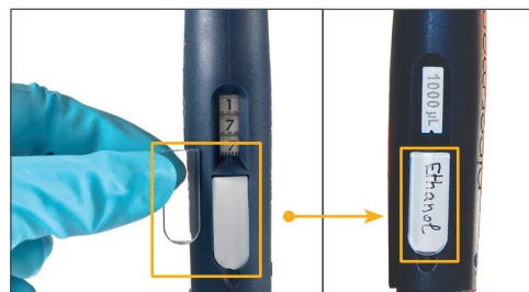
Figure 3 Name tag placement for pipette identification single channel, multichannel, and fixed volume models
